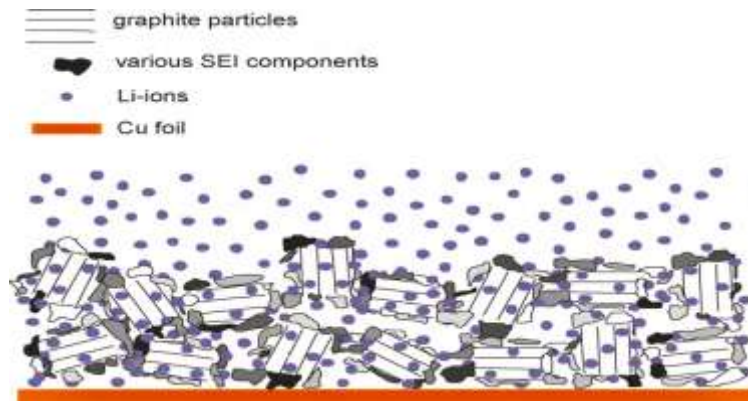
Fig. 4 Sketch of a litigated graphite composite electrode covered by inhomogeneous SEI. The SEI components shown in darker shades of grey are mainly inorganic while those shown in lighter shades of grey are organic
